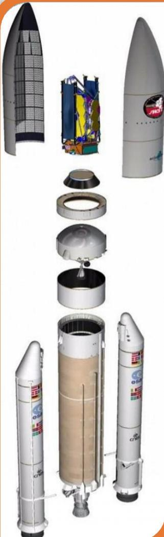
This is the exploded view of a launcher. You can see the satellite inside.
