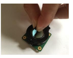
You should start to feel increasing resistance as the filter gets lower. After about nine full turns, the filter should be as low as it can go and you won't be able to turn it any further. Be careful not to over-tighten.
