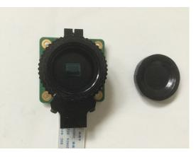
Remove the C/CS adapter ring from the high-quality camera.
