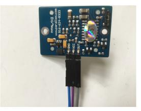
Now we are going to connect each pin on the PIR sensor to an appropriate pin on the Raspberry Pi using the three F-F jumper wires provided in the kit.
