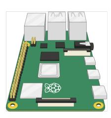
Insert the camera ribbon cable into the Raspberry Pi CSI socket, making sure that the silver side (and not the blue side) is facing the LED matrix. There should be 1 or 2mm of silver still remaining when the cable has been put in correctly.
