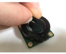
Continue gently turning the filter using the tool. Take care not to touch the glass part of the lens with the tool - it will scratch it.
